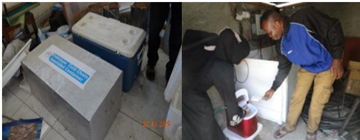
Light-weight insulated container used for storing ice and an ice production unit of the hybrid windmill solar tunnel dryer
